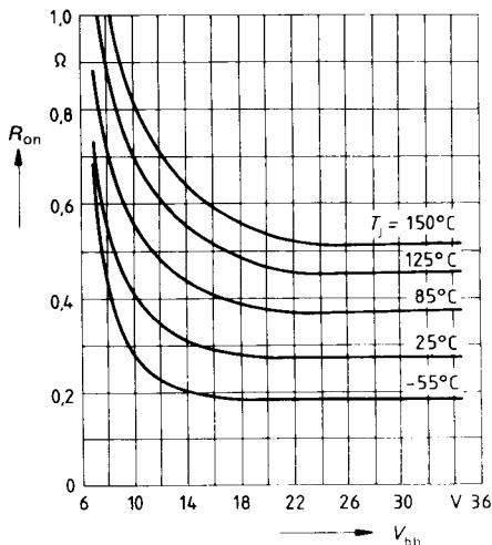
**Typ. short-circuit current  $I_{SC} = f(V_{bb} \text{ and } T_j)$** Parameter:  $R_L = 0.05 \Omega$ ;  $V_{in} = 5 \text{ V}$
