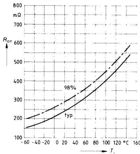
**Typ. drain-source on-state resistance**
