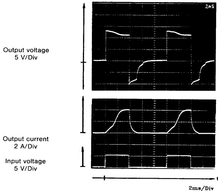
**Figure 3:** Switching with output short-circuited
