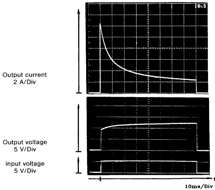
**Figure 2:** Switching a solenoid
