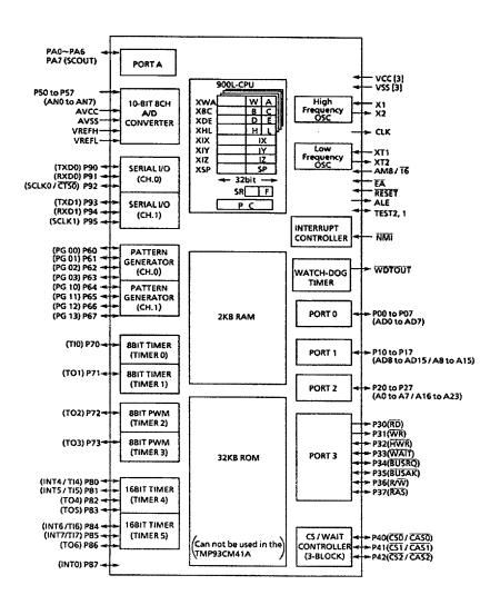
Figure 1. TMP93CM40A/TMP93CM41A Block Diagram
