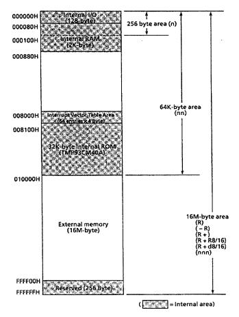
Note: Resetting sets the stack pointer (XSP) to 100H.
