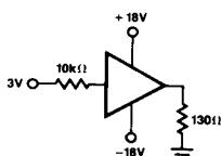
\* **Oil Bath Burn-In:** Use the oil bath heated to +125 °C to provide the heat sink necessary to maintain the junction temperature at < +175 °C.
