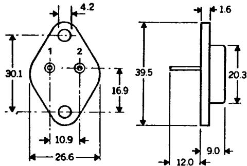
PIN 1—Gate PIN 2—Source CASE—Drain
