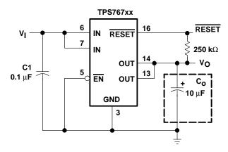
Figure 26. Typical Application Circuit (Fixed Versions)
