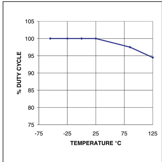
Figure 5. High Drive Maximum Duty Cycle (UC1870-1,-2)
