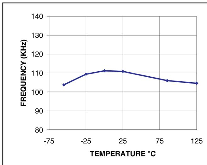
Figure 3. Oscillator Frequency vs. Temperature (CT = 680pF)
