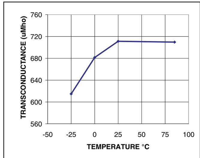
Figure 2. Volt Amp GM (I<sub>OUT</sub> = 10μA)
