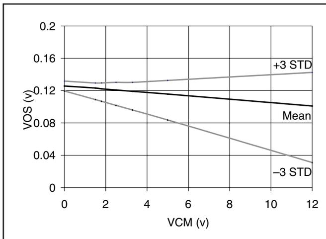
Figure 6. I Limit Voltage Tolerance vs. VCM
