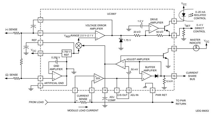
Figure 2. Load System Connection Diagram
