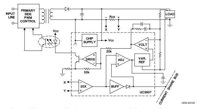
Figure 3. UC3907 In a Load-Sharing Feedback Loop for an Off-Line Isolated Supply
