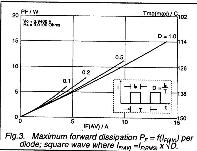
Fig.3. Maximum forward dissipation  $P_F = f(I_{F(AV)})$  per diode; square wave where  $I_{F(AV)} = I_{F(\text{RMS})} \times \sqrt{D}$ .
