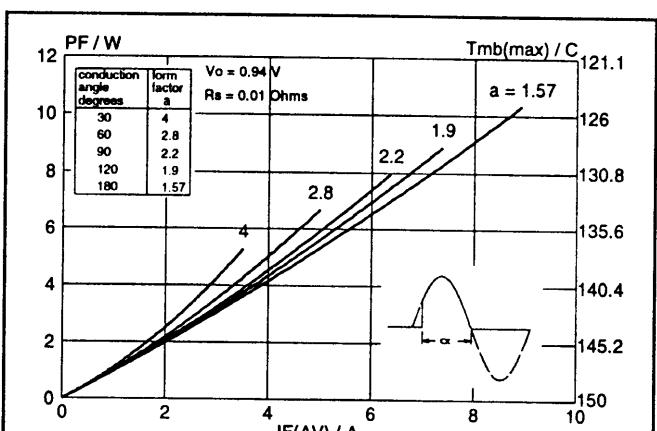
Fig.4. Maximum forward dissipation  $P_F = f(I_{F(AV)})$  per diode; sinusoidal current waveform where  $a = \text{form factor} = I_{F(\text{RMS})} / I_{F(\text{AV})}$ .
