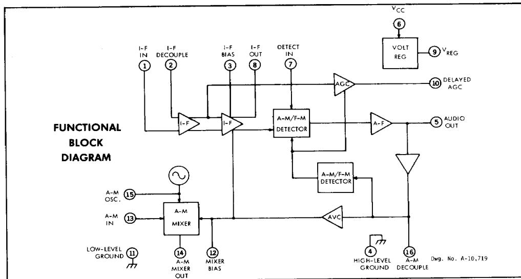
Although primarily intended for use in A-M broadcast reception, the A-M mixer is also suitable for use at long-wave or shortwave frequencies. Delayed AGC is available for use with an optional discrete R-F stage.
