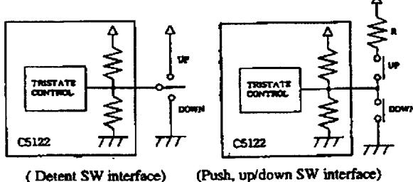
R is a current limiter resistor when both are pressed simultaneously ( $R \leq 1\text{ k}\Omega$ ). In this example, the down operation is performed when both switches are pressed simultaneously.
