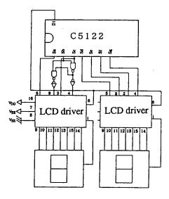
Sa ~ Sc: High-order digit data outputs (BCD) Sd ~ Sg: Low-order digit data outputs (BCD) D1: display drive clock 78 Hz, 50% duty
