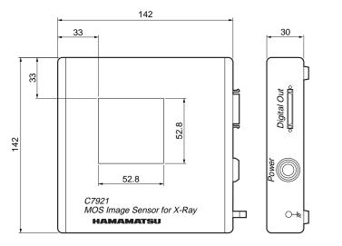
Top cover is made of aluminum 1.0 mm thickness. Weight: 1.37 kg
