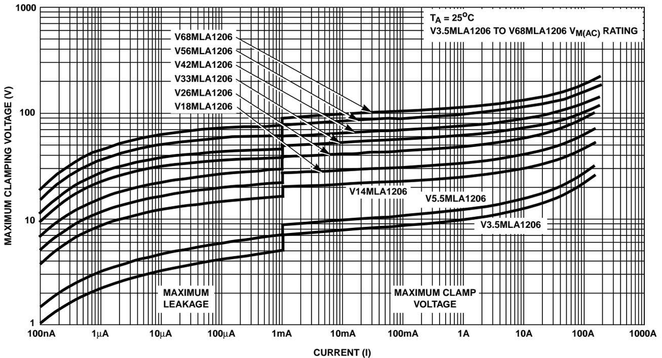
FIGURE 6. V3.5MLA1206 TO V68MLA1206 MAXIMUM V-I CHARACTERISTIC CURVES
