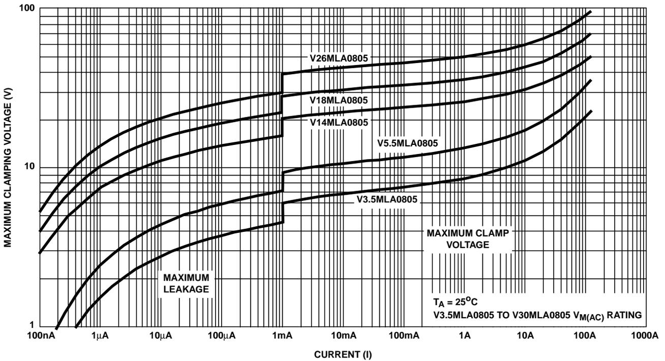
FIGURE 4. V3.5MLA0805 TO V26MLA0805 MAXIMUM V-I CHARACTERISTIC CURVES
