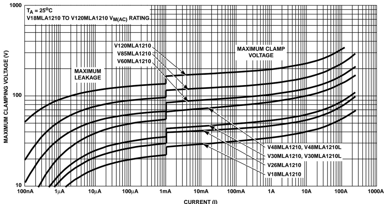
FIGURE 7. V18MLA1210 TO V120MLA1210 MAXIMUM V-I CHARACTERISTIC CURVES
