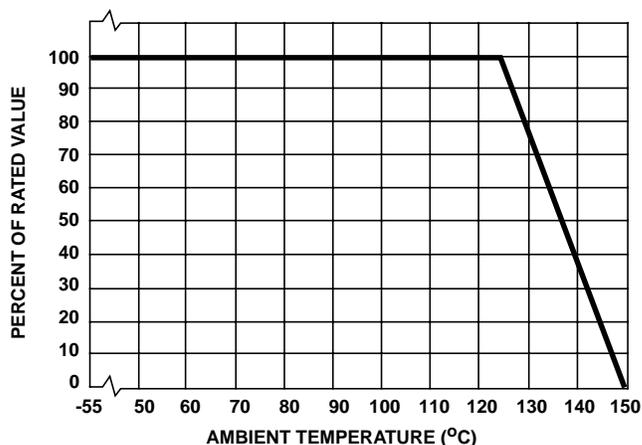
FIGURE 1. CURRENT, ENERGY AND POWER DERATING CURVE
