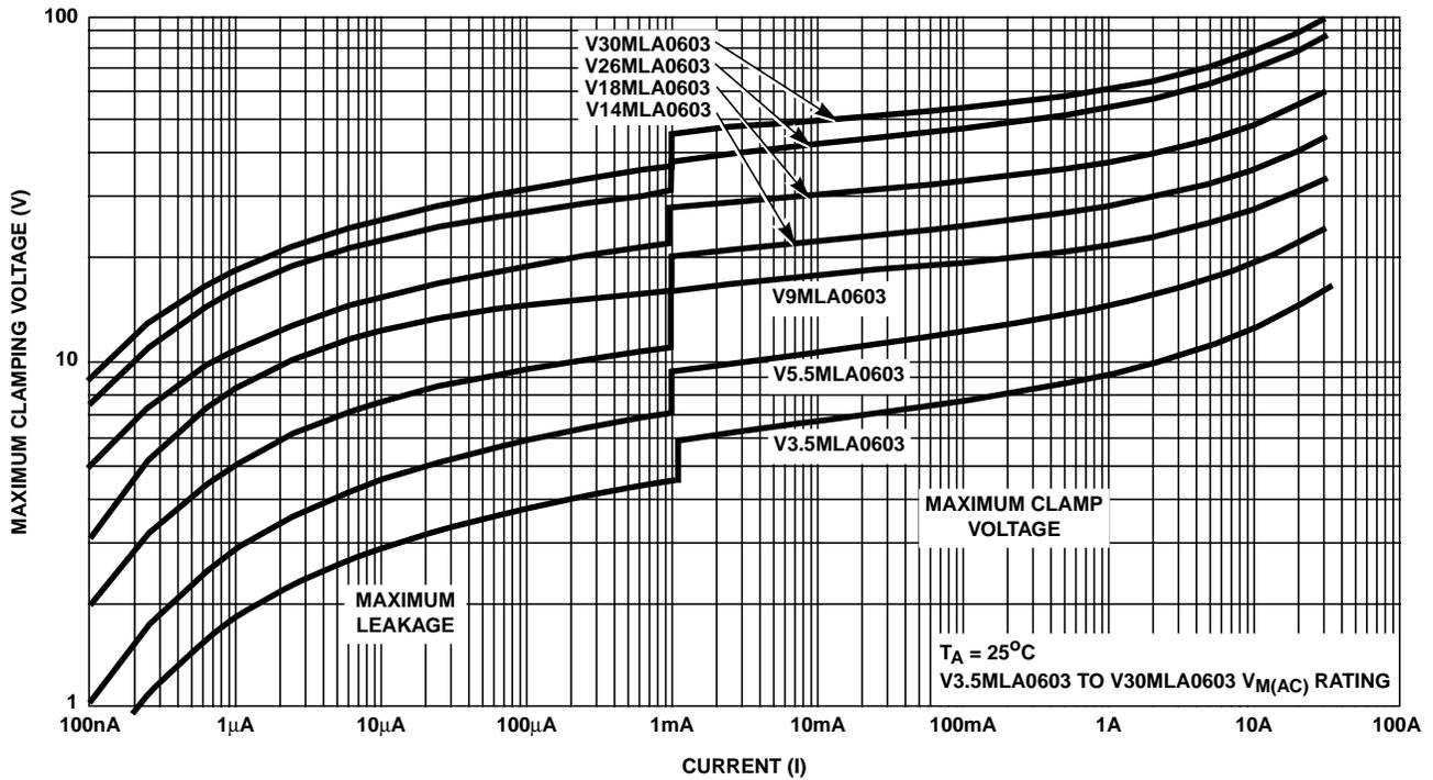
FIGURE 3. V3.5MLA0603 TO V30MLA0603 MAXIMUM V-I CHARACTERISTIC CURVES
