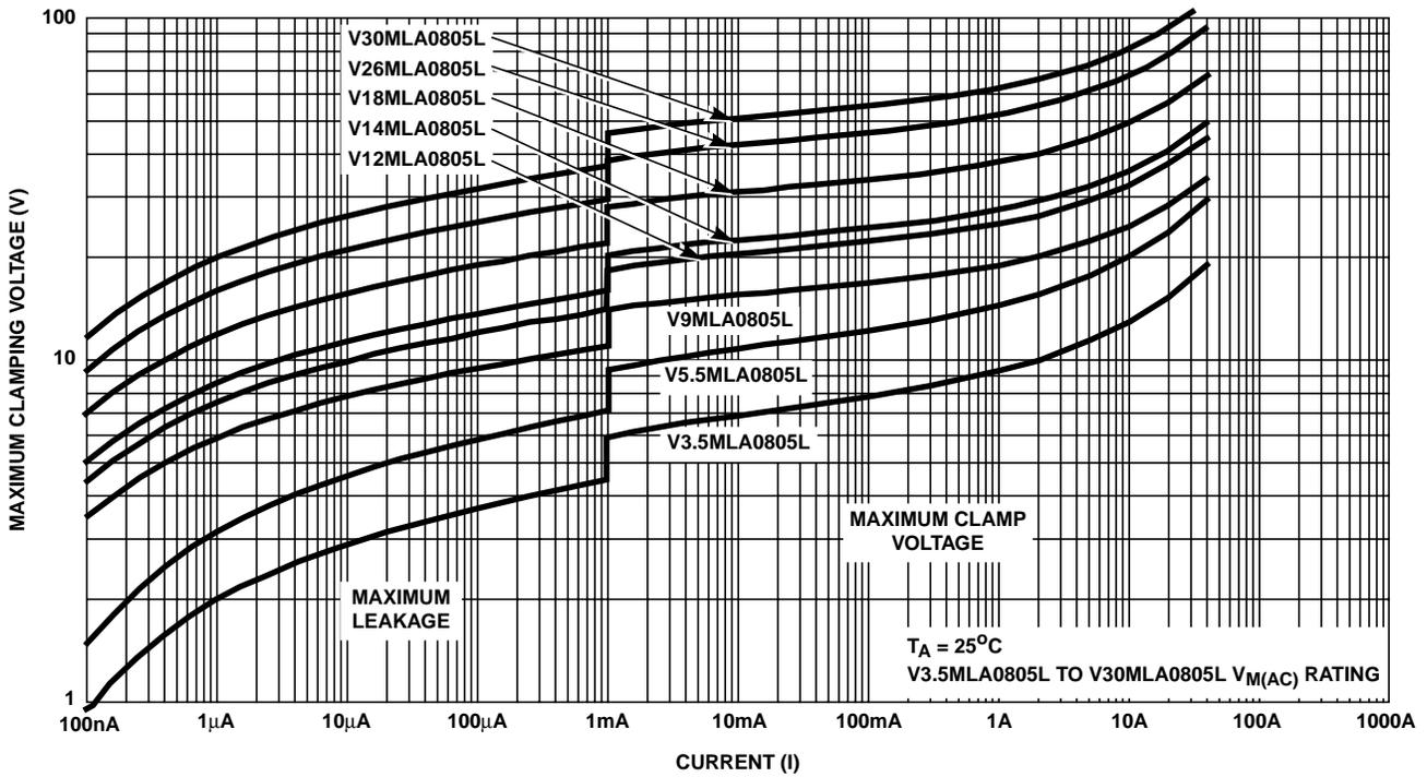
FIGURE 5. V3.5MLA0805L TO V30MLA0805L MAXIMUM V-I CHARACTERISTIC CURVES
