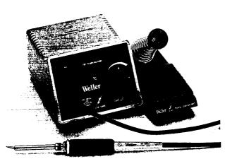
The EC4100M comprises of a EC2100M control unit and an EC1301A miniature soldering iron together with a bench holder with cleaning sponge. This unit offers the same features as the EC2100M with the miniature soldering iron EC1301A. EC1301A soldering iron with standard EPH102 soldering tip. Temperature range of 180° to 450°.
