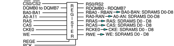
\* Wire per Clock Loading Table/Wiring Diagrams
