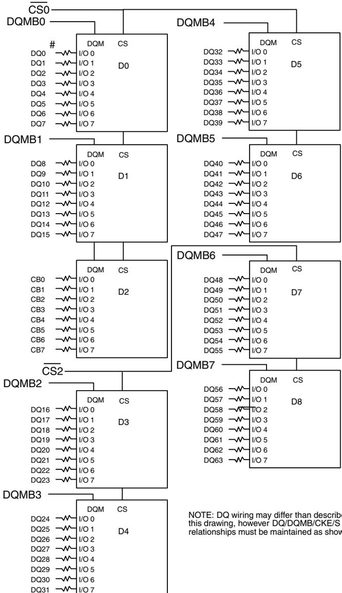
NOTE: DQ wiring may differ than described in this drawing, however DQ/DQMB/CKE/S relationships must be maintained as shown.
