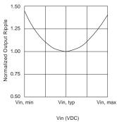
OUTPUT RIPPLE vs INPUT VOLTAGE
