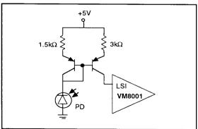
The nominal voltage at the LSI pin is ~ 2Vbe + [ $220\Omega (I_{IN} + 200\mu A)$ ].
