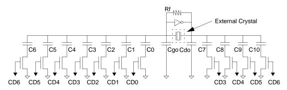
CD = EPROM BIT T = TRANSISTOR C = LOAD CAPACITOR
