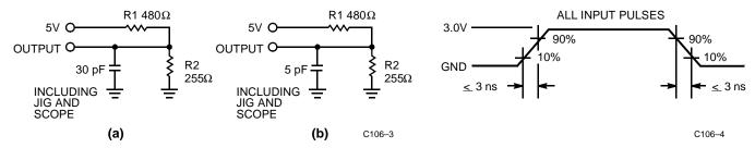
Equivalent to: THÉVENIN EQUIVALENT OUTPUT O  $\frac{167\Omega}{\text{W}}$  O 1.73V
