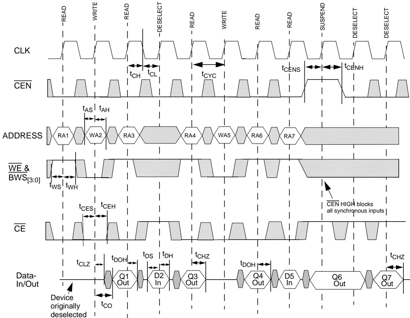
The combination of  $\overline{WE}$  &  $\overline{BWS}_{[3:0]}$  defines a write cycle (see Write Cycle Description table).
