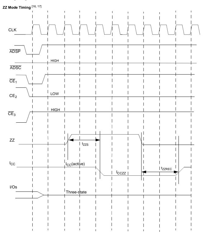
Device must be deselected when entering ZZ mode. See Cycle Description Table for all possible signal conditions to deselect the device.
