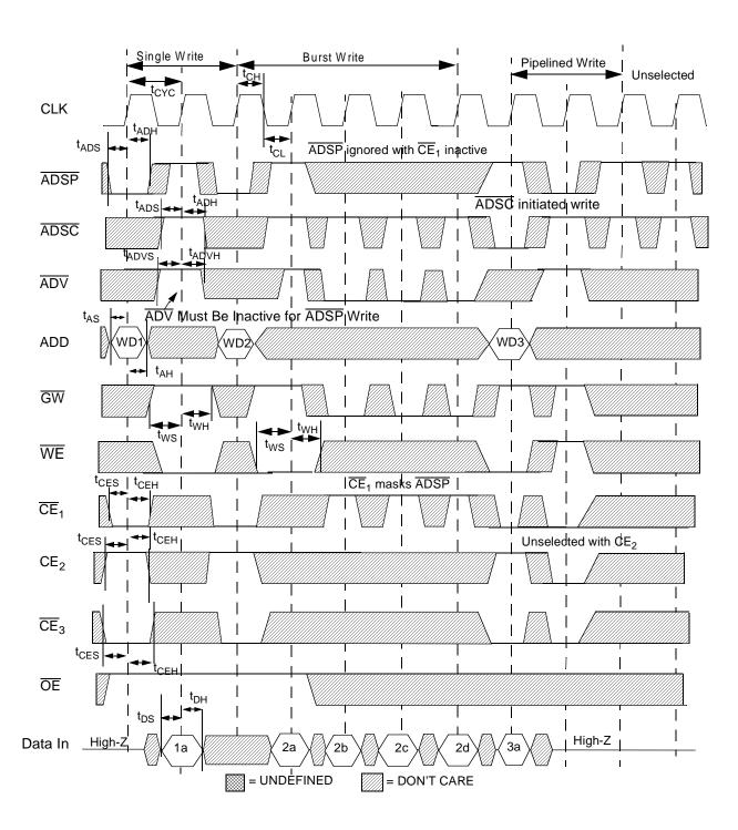
WE is the combination of BWE, BW[3:0] and GW to define a write cycle (see Write Cycle Descriptions table).
