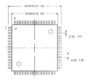
DIMENSIONS IN MILLIMETERS LEAD COPLANARITY 0.102 MAX.
