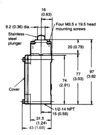
D4B-3171N, D4B-3571N, D4B-3A71N Roller Top Plunger Switch
