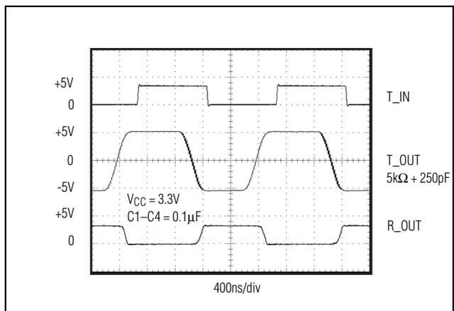
Figure 10. MAX3237E Loopback Test Result at 1000kbps (MBAUD = V<sub>CC</sub>)
