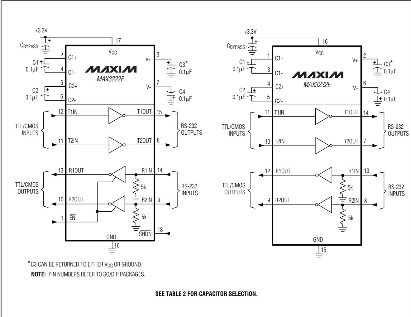
**±15kV ESD-Protected, Down to 10nA, 3.0V to 5.5V, Up to 1Mbps, True RS-232 Transceivers**
