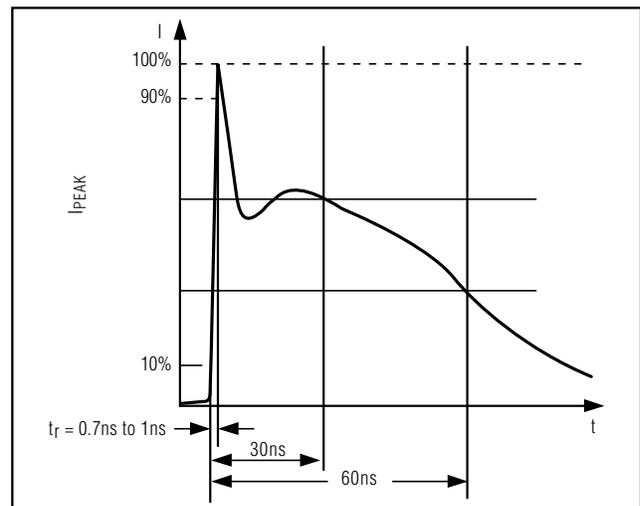
Figure 5b. IEC 1000-4-2 ESD Generator Current Waveform
