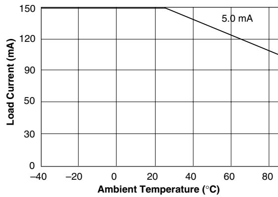
Both relays on with equal load currents.
