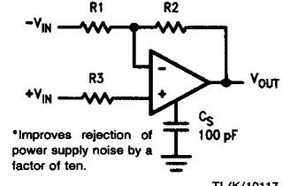
\*Improves rejection of power supply noise by a factor of ten.
