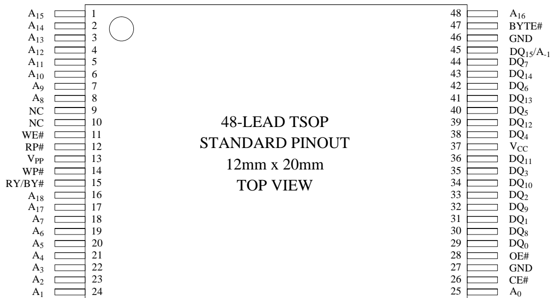
Figure 2. TSOP 48-Lead Pinout
