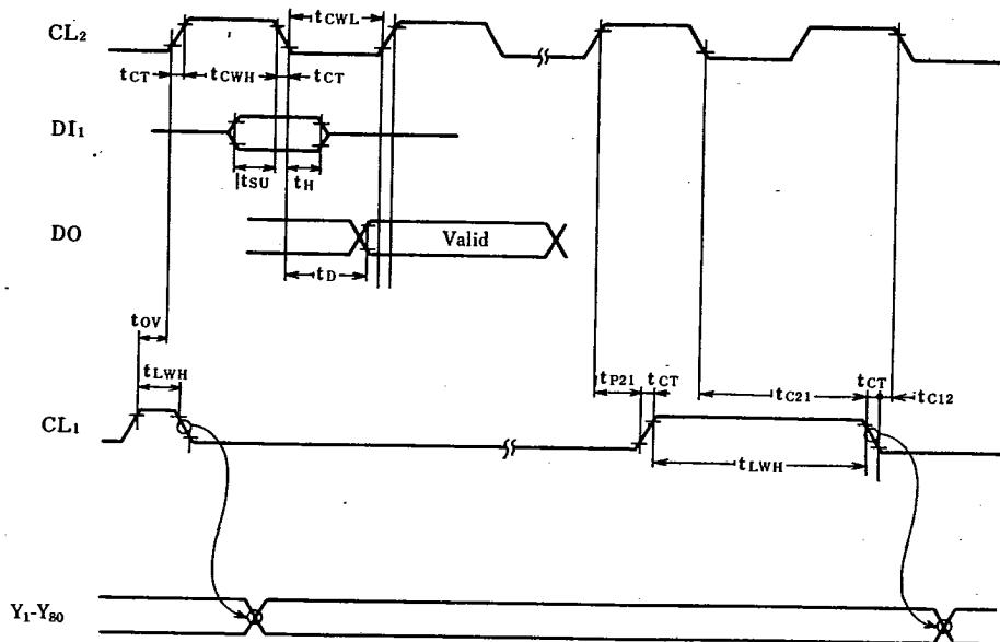
(2) 4-bit Input Segment Driver (PS="High", FCS="Low") ( $V_{DD}=-5V \pm 10\%$ ,  $V_{SS}=0V$ ,  $T_a=-20$  to  $+70^\circ C$ )
