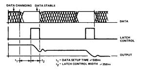
When loading the DAC from an 8-bit computer bus, optimum dynamic response will be obtained when the MSB segment is loaded first, followed by the LSB segments. This sequence allows the MSB's to settle while loading the LSB's. Note that this loading sequence is necessary only when the processor cycle time is longer than the DAC settling time. If
