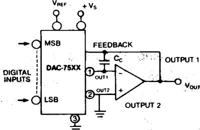
The output amplifier should be selected carefully in order to maintain the dynamic performance of the D/A. In low speed or static applications, AC specifications of the op-amp are not critical. However, in high speed applications slew-rate, settling time, open loop gain and gain/phase margin specifications should be selected for the desired performance.
