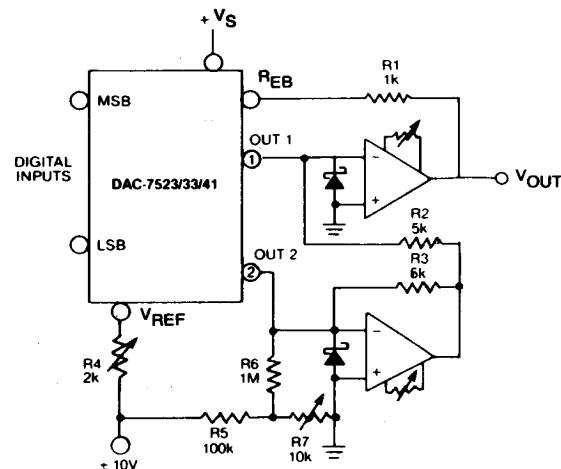
NOTES: R5, R6 and R7 are used to adjust  $V_{OUT} = 0V$  at input 1000.
