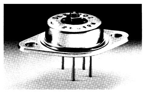
mode, an additional thermal device should be available to provide system shutdown. The Warren G-V Thermulator is powered by a  $\pm 5$ V.DC source, available in most modern systems. The input voltage required should be a low ripple regulated source with a maximum  $\pm 5\%$  tolerance in voltage.
