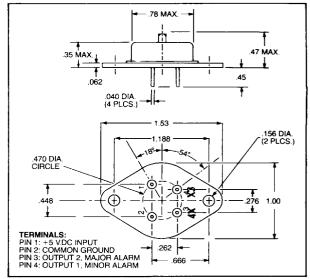
to 55°C upon request. The air velocity factory setting will be established at the selected temperature; differential between the two air velocities could be from 50 to 100FPM. Calibration will be based on the "major alarm" air velocity at the selected air temperature. The "minor alarm" output will track the major alarm setting, at a pre-determined air velocity differential.
