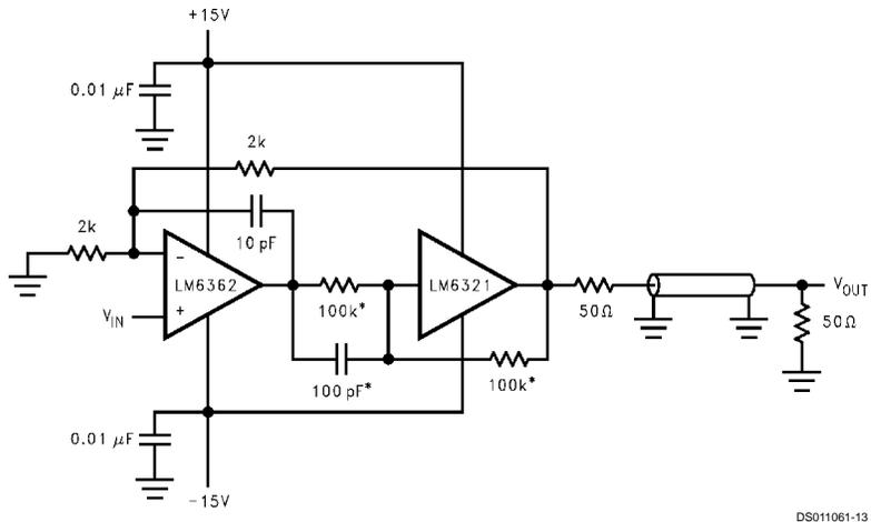
\* Network required when operating on supply voltage over  $\pm 5V$ , for overvoltage protection of LM6321. If  $\pm 5V$  supplies are used, omit network and connect output of LM6362 directly to input of LM6321.
