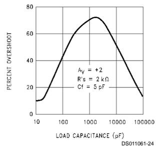
**Typical Performance Characteristics**  $R_L = 10\text{ k}\Omega$ ,  $T_A = 25^\circ\text{C}$  unless otherwise noted (Continued)
