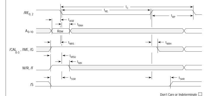
NOTES: 1. All binary combinations of  $A_0$ ,  $A_{2-10}$  must be refreshed every 64ms interval.  $A_1$ does not have to be cycled, but must remain valid during row address setup and hold times.
