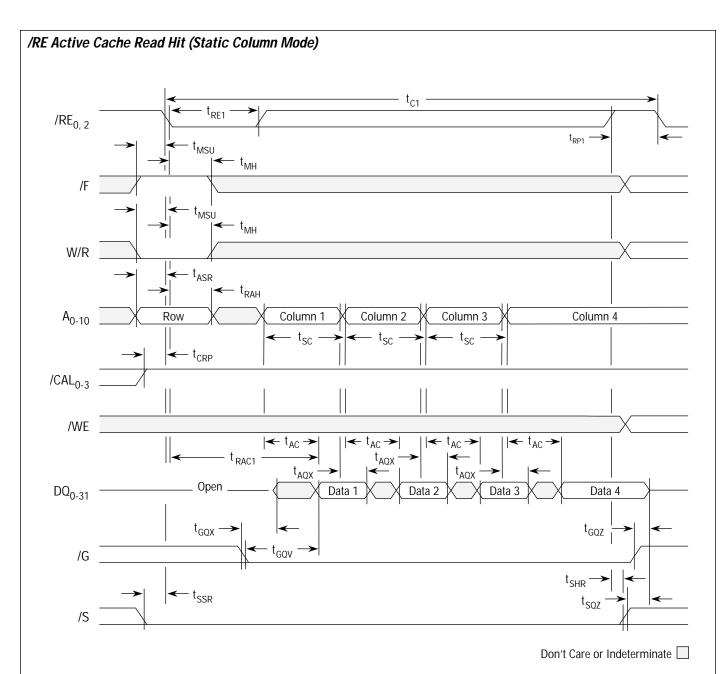
NOTES: 1. If column address 2, 3, or 4 modifies only address pin  $A_0$  or  $A_1$ , then  $t_{AC}$  becomes  $t_{AC1}$  for data 2, 3, and 4, and  $t_{AQX}$  becomes  $t_{AQX1}$  for data 1, 2, and 3.
