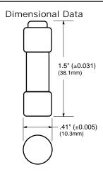
Catalog Symbol: LP-CC Time-Delay, Current-Limiting Ampere Rating: ½ to 30 Amperes AC Voltage Rating: 600 Volts (or less) Interrupting Rating: 200,000A RMS Sym.
