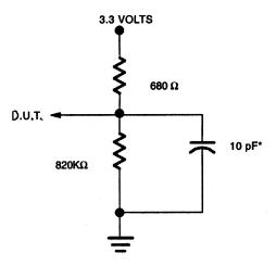
\* INCLUDING SCOPE AND JIG CAPACITANCE
