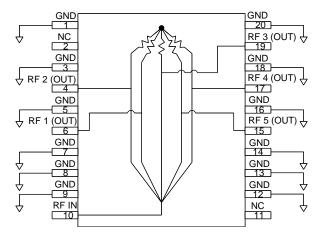
Pins labeled as ground should be DC and RF grounded.
