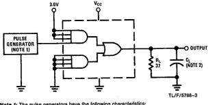
Note 1: The pulse generators have the following characteristics:  $Z_{OUT} \approx 50\Omega$ ,  $t_W = 200$  ns, duty cycle = 50%,  $t_{r_1} = t_f = 5.0$  ns. Note 2: CL includes probe and jig capacitance.
