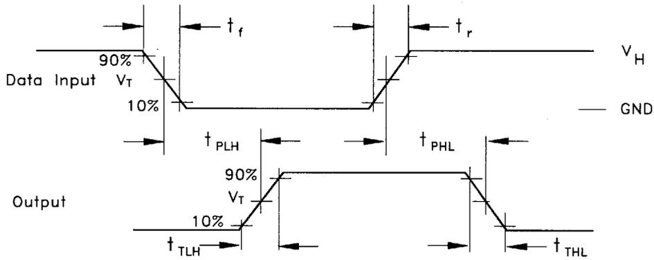
Input and Output Threshold Voltage: V<sub>T</sub> = 50% V<sub>CC</sub> for HC,
