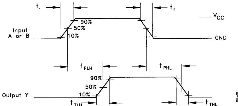
Input and Output threshold voltage, V<sub>T</sub>=50% V<sub>CC</sub> for HC; 1.3V for HCT
