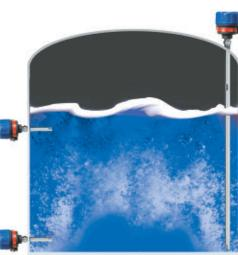
Challenging process conditions such as suspended solids or aeration are best managed with pulsed-signal technology. Models 961/962 switches further minimize the effects of mild turbulence or splashing with adjustable time delays.
