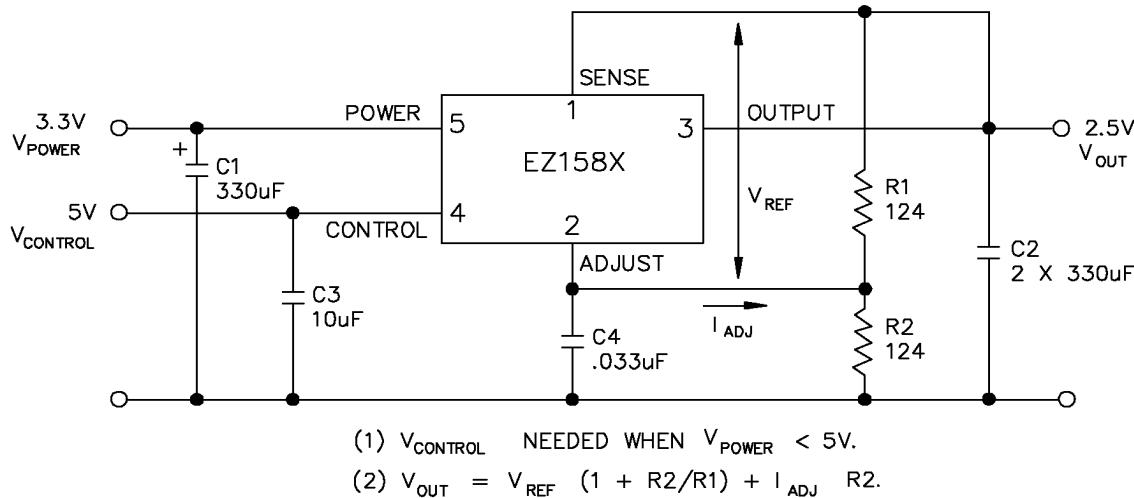
**Flexible Motherboard Design, using the EZ158X and EZ1900 Regulator Balance Controller**
