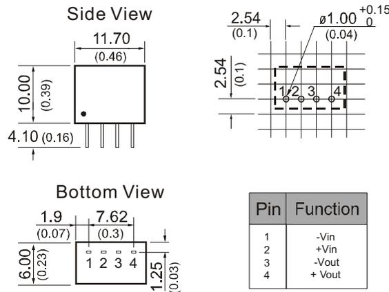
Note: All Pins on a 2.54mm(0.1) pitch; All Pin diameters are 0.50 mm(0.02);
