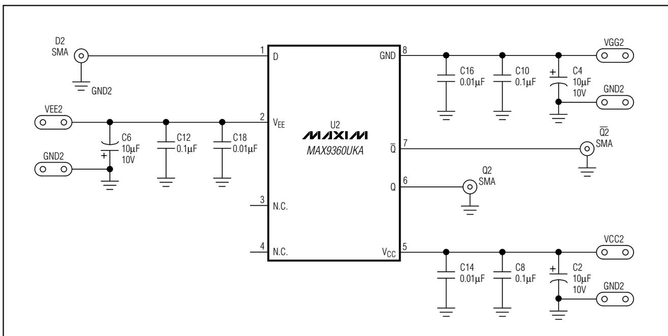
Figure 2. MAX9360 EV Kit Schematic (MAX9360UKA Circuit)
