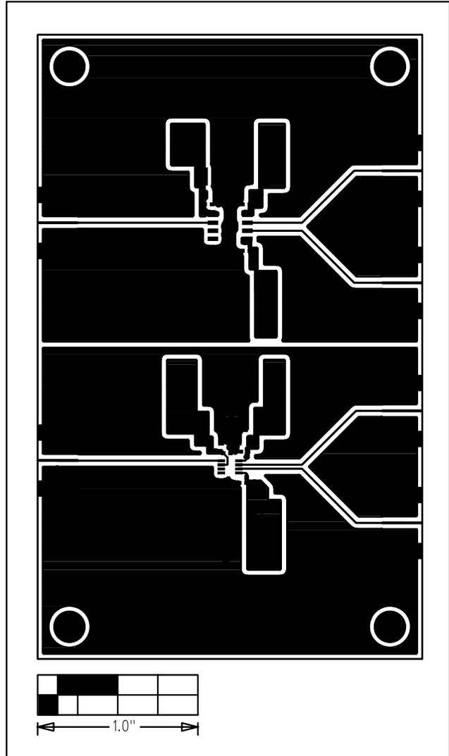
Figure 4. MAX9360 EV Kit PC Board Layout—Component Side
