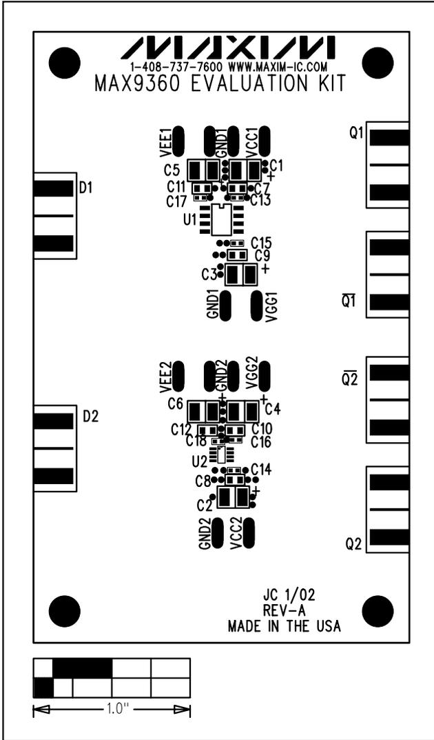
Figure 3. MAX9360 EV Kit Component Placement Guide—Component Side
