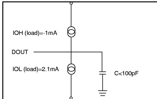
Note: No output loading is present in tester load board.
