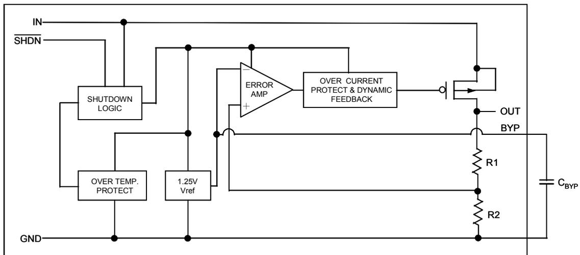
Figure 1. Functional Diagram
