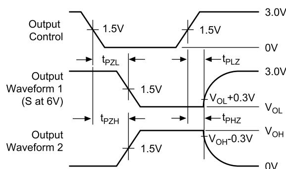
Waveform 1 is for an output with internal conditions such that the output is low except when disabled by the output control.
