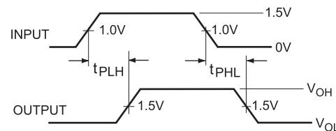
All input pulses have the following characteristics: frequency = 10 MHz,  $t_p = 4 = 2\text{ns}$ ,  $Z_O = 50\Omega$ . The outputs are measured one at a time with one transition per measurement.
