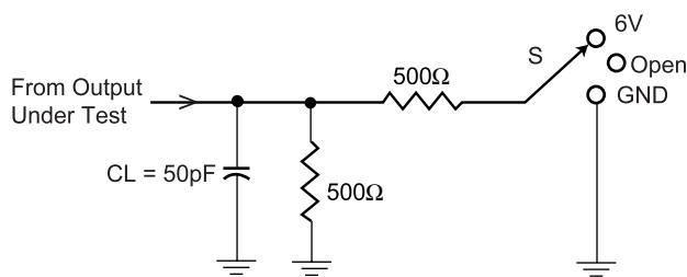
CL includes probes and jig capacitance.
