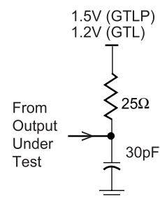
CL includes probes and jig capacitance.
