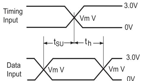
All input pulses have the following characteristics: frequency = 10 MHz,  $t_r = t_f = 2\text{ns}$ ,  $Z_O = 50\Omega$ . The outputs are measured one at a time with one transition per measurement.
