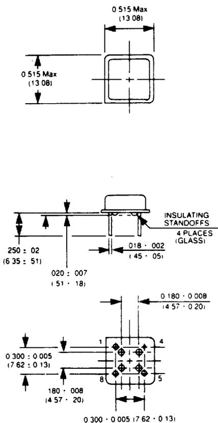
Pin number 4 connected to case.
