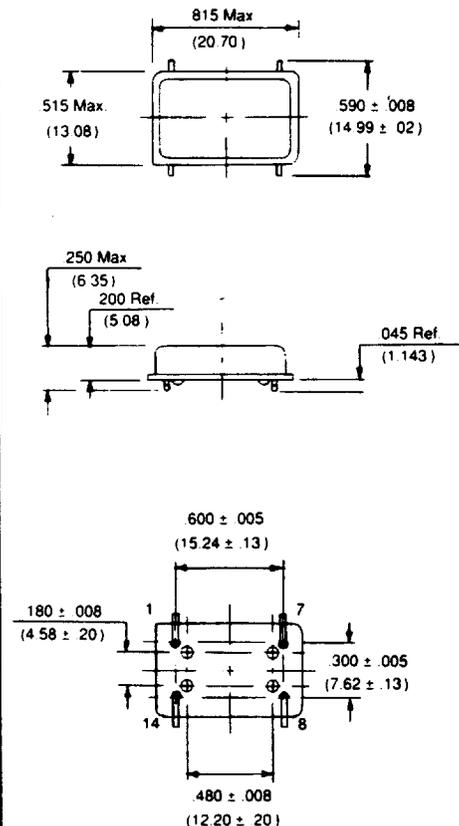
Pin number 7 connected to case.
