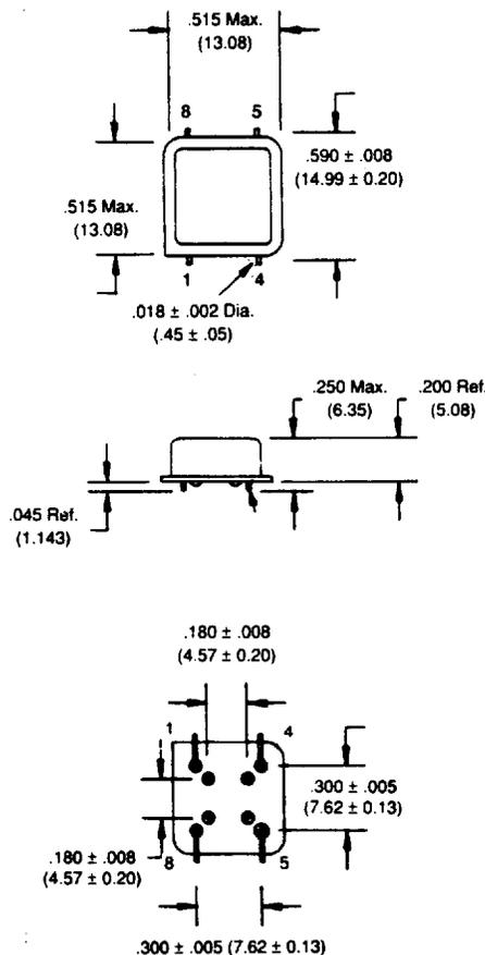
Pin number 4 connected to case.
