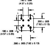
Pin number 4 connected to case. Seating plane = .005 Max. (.127) Wire leads to be formed to a 90° angle. SM Series
