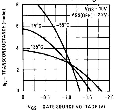
**Transconductance vs. Gate Source Voltage**
