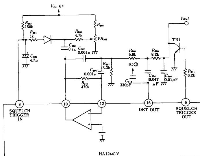
Notes: Connect C119 to V<sub>cc</sub> line as near to Pin 13 as possible.
